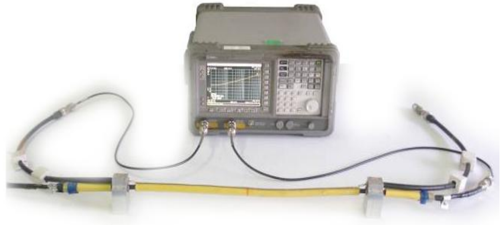
Cable Surface Transfer Impedance measurement setup
